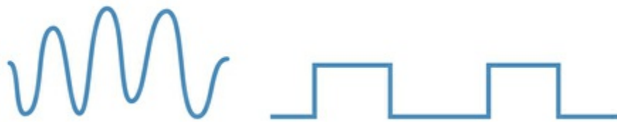
FIGURE 3.2 An analog signal and a digital signal
