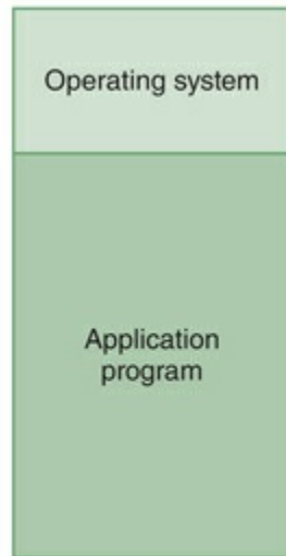
FIGURE 10.5 Main memory divided into two sections
