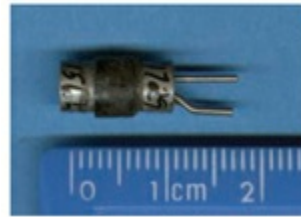
FIGURE 1.7 A transistor, which replaced the vacuum tube Courtesy of Dr. Andrew Wylie
